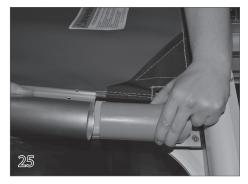
Slide the nylon leading edge inserts into the ends of the leading edge tube. Note, one of these insert assemblies is in the track while the other is outside of the track. Make sure the inserts can slide freely inside the leading edge tube. If they don't, clean off any burrs that may be causing them to bind.
