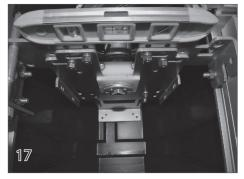
With the brackets on the non-motor end in position, place a small level across the brackets to make sure they are level. Tighten the 4 mounting arm bolts on the adjustable brackets.
