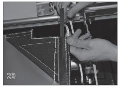
Apply the supplied grease to the magnet. This will help it slide in the webbing easier. Slide the magnet (31) into the webbing with the same side facing up that shut the motor off when it was passed in front of the sensor.
