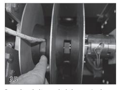
Press the tab down to lock the rope in place.
