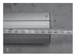
To determine if the cover system was ordered correctly for the pool, the length of the roll-up tube should be 6 inches shorter than the track space.
