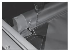
Drill a 3/32" pilot hole through the top of the rope channel of the leading edge tube. Do this on both ends of the leading edge tube.
