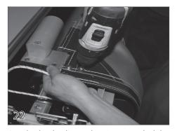
Attach the leading edge insert and slider plate to the cover by threading (2)  $4-20 \times 5/8''$  two screws (32) and the  $1/4 \times 5/8''$  washers (34) that come attached to the slider plate, through the pre punched holes in the cover and into the slider plate. Repeat this on both sides of the cover. Use caution if using a drill to attach these screws.
