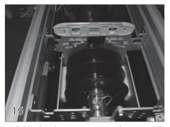
With the brackets in position, place a small level across them to make sure they are level. Place the small level on the motor to make sure it is level. If the motor isn't level, it may affect the shifting of the drive mechanism. Tighten the eight nuts on the adjustable motor end brackets.
