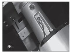
Attach the bond wire from the tail of the cover to the bonding lug (37) that is attached to the end casting.
