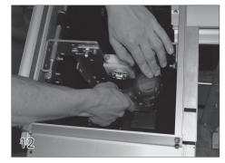
Anchoring the Mechanism Feet With the mechanism centered between the tracks and centered in the cover box front to back, anchor the mechanism mounting feet into the cover box. Use the appropriate screws and anchors depending on the type of cover box being used.
