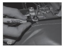
With the cover in the fully closed position, mark the webbing where it is in line with the sensor that is mounted on the guide.
