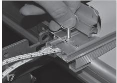
Insert the locking ring pin (25) through the retainer and the track. This will lock the track into the retainer so it can't slide into the cover box as the cover system is operating.
