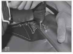
Position the fabric on the leading edge so it is in line with the edge of the rope C-channel. Pin the rope hem to the leading edge by placing a #10 x 5/8" pinning screw (43) in the drilled hole and through the rope hem. Do this on both ends of the leading edge bar.
