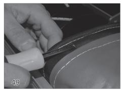
Insert a screw driver through the slit in the webbing to create the pocket for the magnet.
