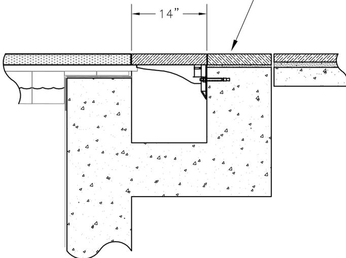
If using stones wider than housing, finish deck short and support back of stone with mortar
