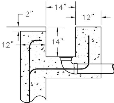
Because coping and deck thickness vary, housing depth is always measured from the top of beam or top of encapsulation.
