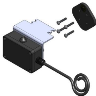
Rotary Encoder Limit Switch
