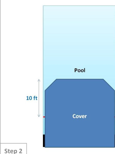
The diagram shows a cross-section of a pool and its cover. The pool is light blue and the cover is dark blue. A red horizontal line is drawn across the pool, indicating the 'Home' position. A vertical double-headed arrow to the left of this line is labeled '10 ft', indicating the distance from the top of the pool to the 'Home' position. The cover is shown fully closed, with its top edge aligned with the 'Home' line.
