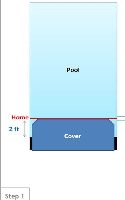
The diagram shows a cross-section of a pool and its cover. The pool is light blue and the cover is dark blue. A red horizontal line is drawn across the pool, labeled 'Home' in red. A vertical double-headed arrow to the left of this line is labeled '2 ft', indicating the distance from the top of the pool to the 'Home' position. The cover is shown partially open, with its top edge aligned with the 'Home' line.
