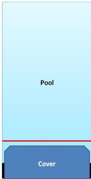
Operate cover in the **open** direction until the cover has gone 6 in. to 1 ft. past the home position.
