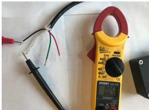
Using a multi-meter set to **Ohms ( $\Omega$ )**, place one probe on the **white** wire from the Rotary Encoder and place the other probe on the **black** wire from the Rotary Encoder.
