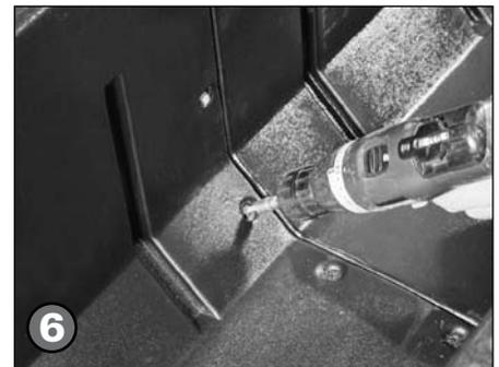
6 Fasten the sections together from the inside of the housing to the outside with six 1" tek screws. Repeat this process to assemble the full length of the polymer housing.
