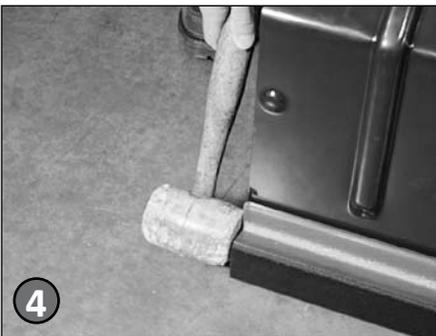
4 Use a rubber mallet to tap the sections together if necessary.
