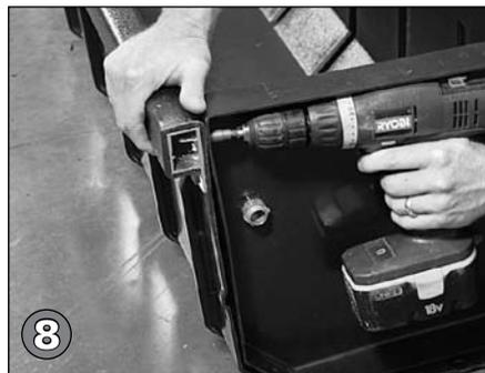
8 Now fasten end piece into place using eight 1" tek screws. To do this, position the end piece flush with the side wall of the housing and fasten one tek screw into each top rail as shown. All other screws should be fastened from the outside of the housing pointing in. Fasten the other box end (4, M9344) into place in the same manner on the opposite side of the housing.
