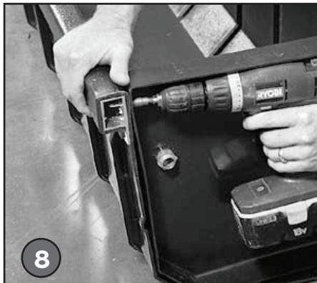
Now fasten end piece into place using eight 1" tek screws. To do this, position the end piece flush with the side wall of the housing and fasten one tek screw into each top rail as shown. All other screws should be fastened from the outside of the housing pointing in. Fasten the other box end (4, M9344) into place in the same manner on the opposite side of the housing.
