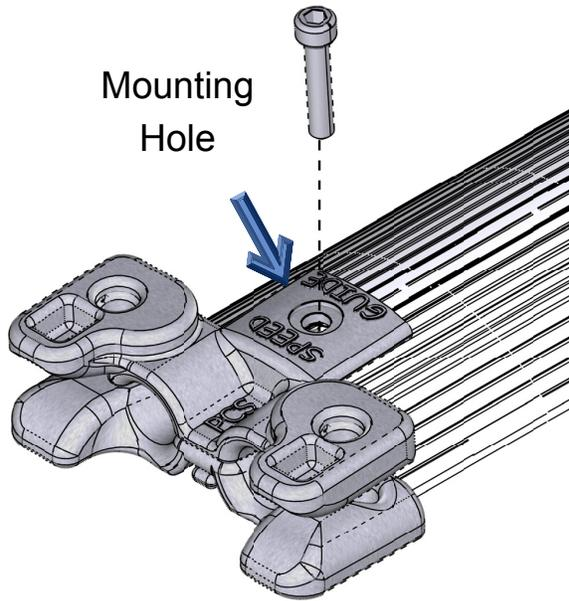
6. Use the 5/16" allen head bolt to secure the guide to the tracks.
