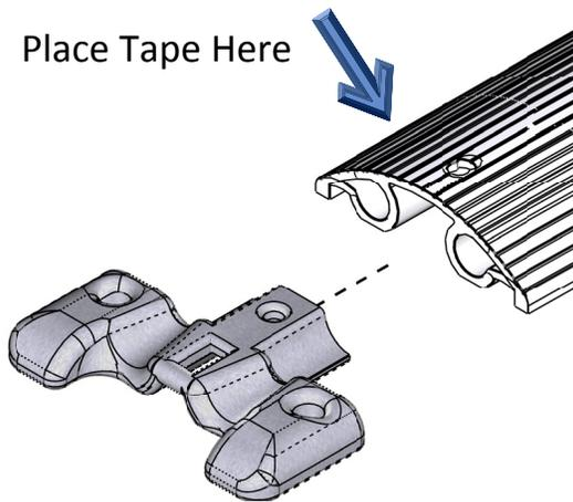
2. Place the nut in the keyed groove. Slide the bottom piece into the center channel of the track.
