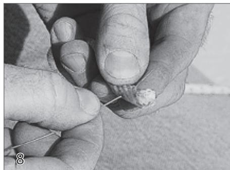
**Alternate Rope Feeding Method** Another common method of running rope in the track is to pierce the rope with a small piece of wire. This wire then becomes the pulling handle as you feed the rope into the end of the track. This is especially useful if retainer isn't being used and the tracks are already installed.
