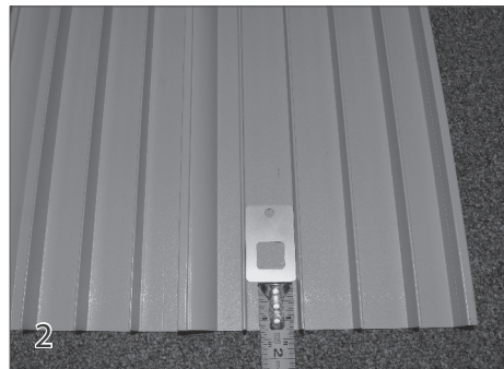
Insert the lid lock backing plate between two ribs on the underside of the lid panel. Position the plate so it is 1-1/4" from the end of the lid panel.
