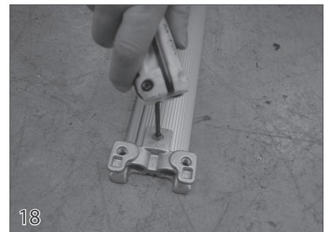
Insert the guide on the end of the track at the mechanism end. The bottom half of the guide is keyed to hold the nut in place. Using a 5/32" allen wrench, tighten the screw on the top of the guide (12).
