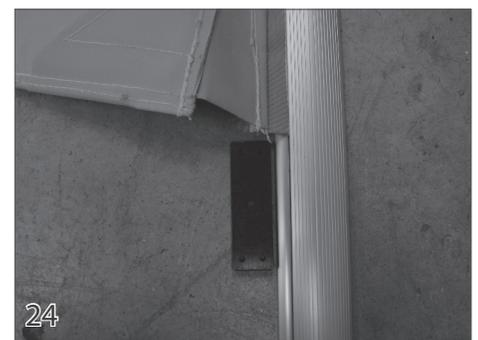
24 Press the beveled side of the bottom half of the positive stop (34) against the inside edge of the cover. Slide it underneath the cover. The holes in the positive stop should line up with the holes in the cover.
