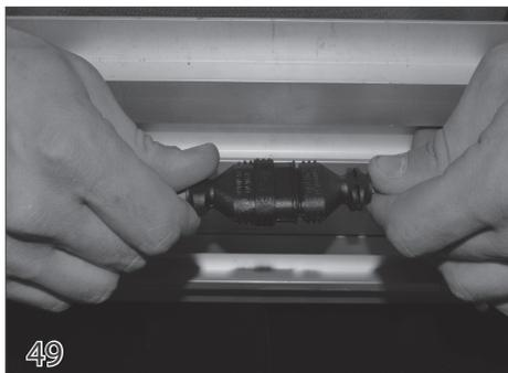
Connect the sensor wire to the motor wires by pressing the wire connections together.
