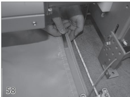
58 Insert the magnet (18) through the slit in the webbing. Continue pushing the magnet forward until it is completely inside the webbing and in line with the mark on the webbing.
