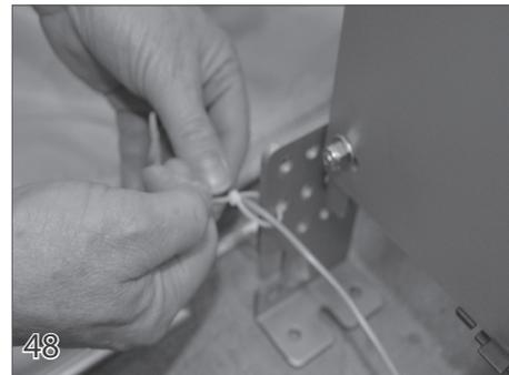
Use cable ties (22) to secure the sensor wire to the motor end of the mechanism to keep it secure and from getting caught in the cover or ropes.
