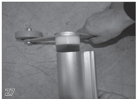
27 Insert the wheel assembly (6) into the leading edge.
