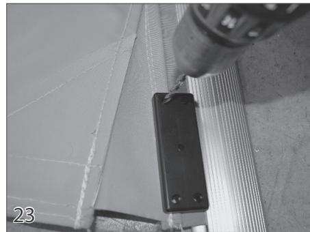
23 Position the top half of the positive stop (33) over the webbing of the cover. Use it as a template to drill through the holes in the positive stop and through the webbing of the cover. Remove the positive stop.
