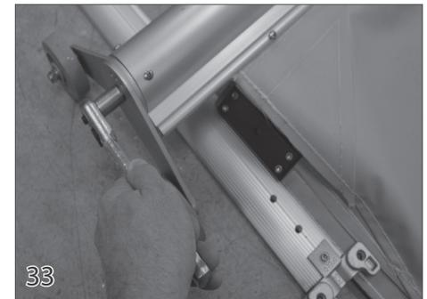
Adjust the height of the wheel assembly so the leading edge will clear any obstacles near the pool such as slides and hand rails. Repeat this step on the opposite side of the cover.
