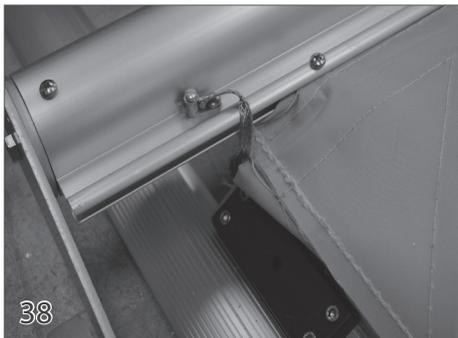
Connect the bonding wire that is attached to the front corner of the cover to the leading edge tube by first securing a bonding lug (24) to the bar, using the 10 - 32 x 1" screw (21) and 10-32 nylock nut provided (27). Then, insert and tighten the bond wire in the bonding lug. Do this on both sides of the leading edge tube.
