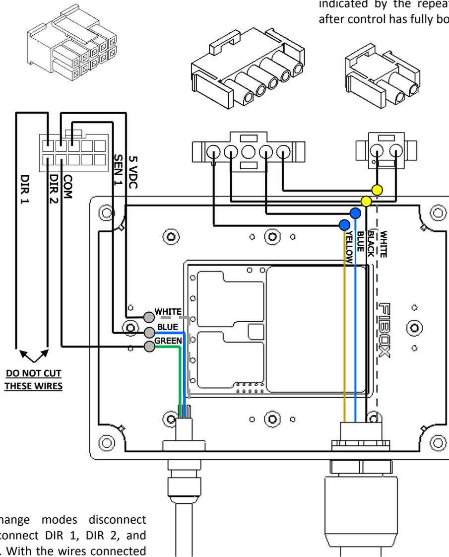
**NOTE:** To change modes disconnect power, then connect DIR 1, DIR 2, and COM together. With the wires connected reconnect power. Once the LED flashes blue disconnect the wires. This will cycle through the modes.
