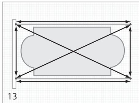
Lengths, widths and diagonal dimensions must be equal to each other or the system will not operate properly.
