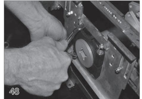
The non-motor brake should be tight enough to prevent the cover from rolling off the tube faster than it is being pulled into the track. To adjust this brake, use two 7/16" wrenches and tightening or loosening the thru bolts in the brake block.
