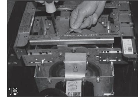
On the motor and non-motor side, use the half inch screws and nylock nuts provided and bolt the cross braces together.
