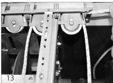
Insert the rope from the non motor end into the channel behind the first pulley on the motor end. Push the rope behind all three pulleys and out of the channel behind the third pulley.
