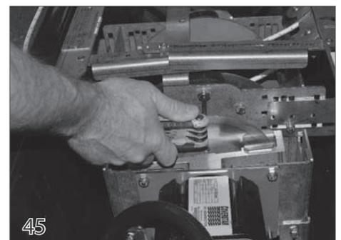
To tighten the brake, use an allen wrench to turn the set screw inside the jam nut in the clockwise direction.
