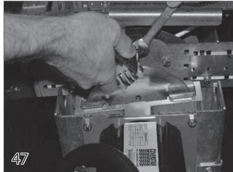
After adjusting the set screw, retighten the jamb nut while holding the set screw with an allen wrench. There's a corresponding brake on the opposite side of the rope reel. Adjust both brakes equally.
