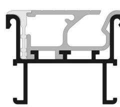
Recessed Horizontal track with Track, Housing and Spacer
