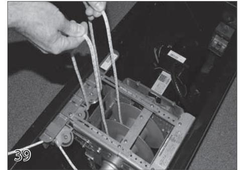
If both ropes are the same length, and the cover doesn't close squarely, shorten the rope for the side of the cover that doesn't close all the way. The amount that the rope is shortened is equal to the amount distance that the cover needed to travel to close all the way. While holding the rope, run the switch in the cover position.
