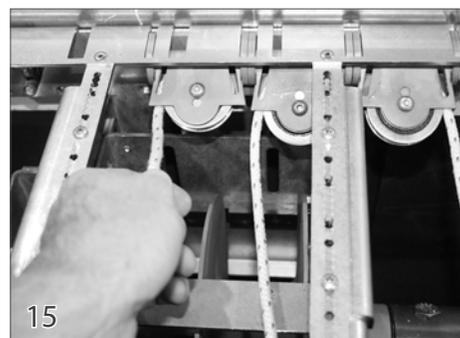
Continue pulling the excess rope through the pulleys.
