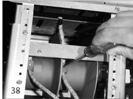
If one of the ropes is longer than the other rope, loosen the set screw that secures the rope to the rope reel lug. Shorten this rope until it is the same length as the other rope. Re-attach the rope to the rope reel.
