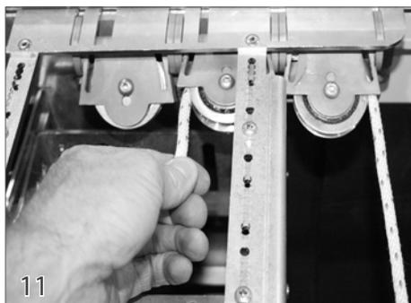
Insert the rope into the side of the first pulley. Push the rope behind that pulley and out along the side of the second pulley.
