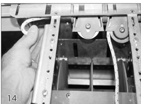
Bend a curve into the end of the rope and pull it back just until it is in the middle of the pulleys. Now push the rope back until it comes out the side of the third pulley.
