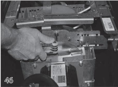
To loosen the brake, use an allen wrench to turn the set screw inside the jam nut in the counter clockwise direction.
