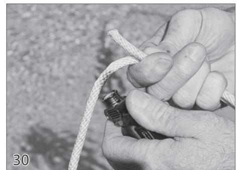
Pull both ropes until the leading edge just moves on each side, cut the longer rope to the same length as the shorter rope while tight. These ropes should be at least 8ft long. Use a lighter or torch to burn the ends of the rope. In most cases you will only need to cut one rope.
