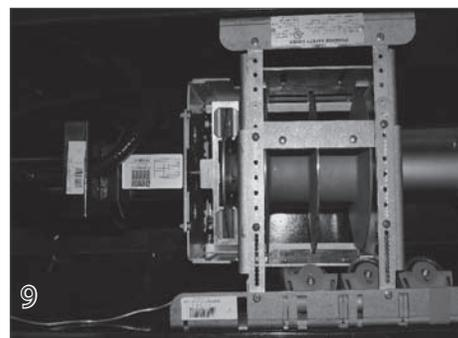
Position the mechanism in the housing so that the roll-up tube is centered in the housing and the first pulley is properly aligned with the track.
