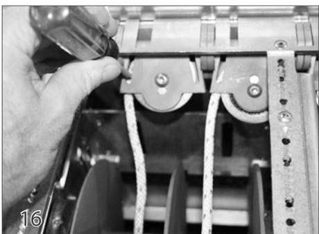
To help guide the rope around the pulleys, inset a small screw driver into the slots in the pulley housings.
