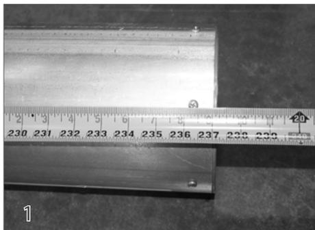
To determine if the cover system was ordered correctly for the pool, the length of the roll-up tube should be 3 inches shorter than the track space.
