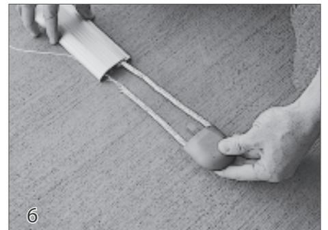
Feed the rope through the pulley assembly (27) and place the pulley housing onto the end of the track.
