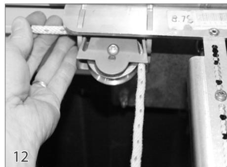
On the non-motor end, run the rope around the pulley and out the back channel of the pulley assembly. Pull this rope along the backside of the cover housing to the motor end pulley assembly.
