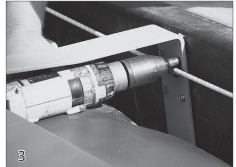
Secure the brackets to the back wall of the housing using #12 x 1-1/2" hex head sheet metal screws. Mount a rope loop on one top screw of each of the brackets. This will keep the rope running straight along the back of the housing.
