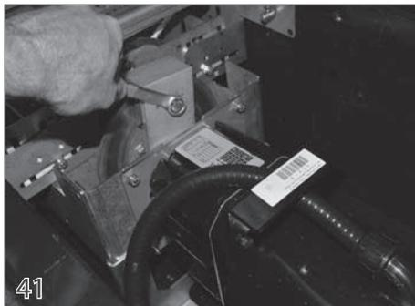
To adjust the torque limiter, use the provided 9/16" wrench attached to the mechanism to tighten the first brake bolt 1/2 turn. Run the cover.
