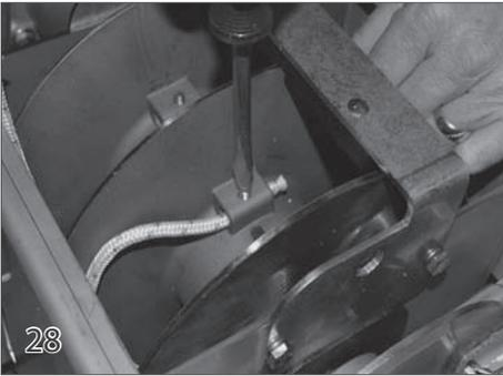
**Attaching the Ropes to the Rope Reel**
