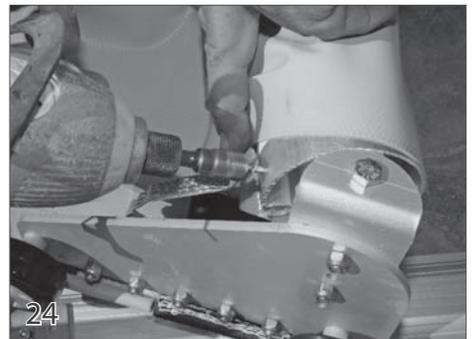
Connect the bonding wire that is attached to the front corner of the cover to the leading edge bar using a tek screw. Be sure the screw doesn't interfere with the leading edge insert.
