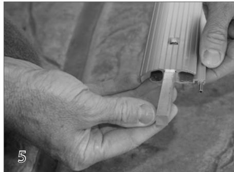
Tap the spring pin (31) into the round splice channel. Slide the center splice (30) into the center channel.
