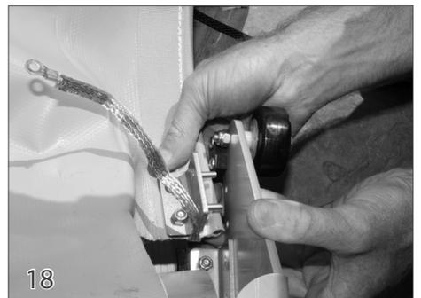
Connect the two hole bracket that is attached to the front corners of the cover to the wheel assemblies.
