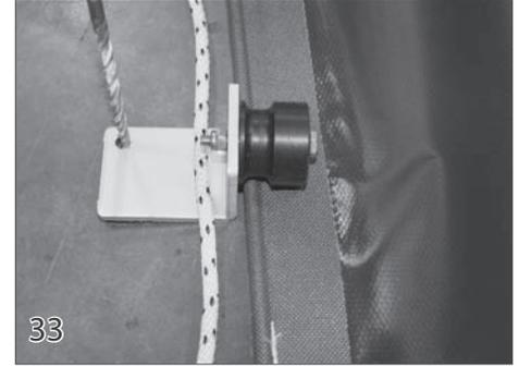
To help the cover roll up evenly, install a cover roller (37) 2-3 inches behind the guide feed. Secure the cover roller to the deck using the screws (15) and anchors (25) provided.
