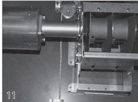
11 Align the mechanism on the motor side first by using a piece of rope. Extend it from the outside channel of the track to the pulley to make sure the rope will feed directly into the pulley.
