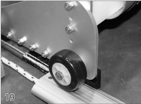
Feed the wheel assembly (8) and cover into the track.
