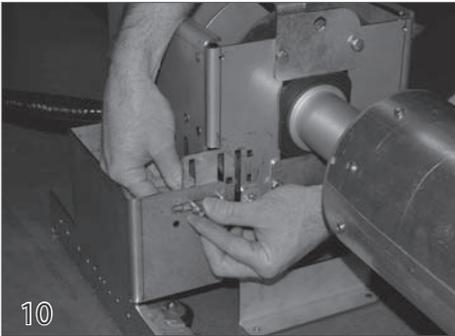
10 Use a 7/16" wrench to tighten the nylock nuts. Additional carriage bolts (27) and nylock nuts (29) are provided and can be used as reinforcement for the pulley brackets as needed.
