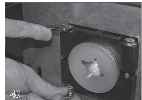
To loosen the brake, use an allen wrench to turn the set screw inside the jam nut in the counter clockwise direction.
