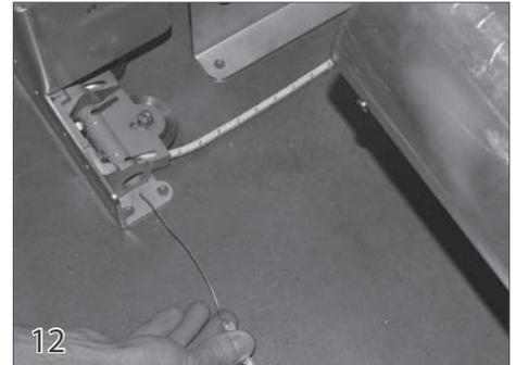
Insert the wire that is attached to the rope end into the channel behind the first pulley. Continue to push the wire until it comes out of the channel behind the third pulley.
