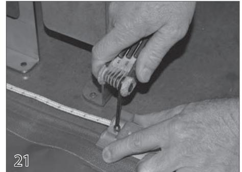
Use a  $5/32$  allen wrench to tighten the screw that connects the two sections of guide feed together.
