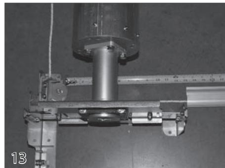
13 On both the motor end and non-motor end of the mechanism, measure from the cover track to the pulley. It is important that the mechanism be mounted square to the cover track.
