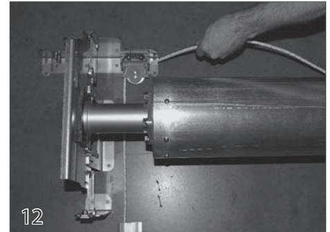
12 Go to the non-motor end and make sure the rope will come straight back from the rope channel of the track to the pulley. If the ropes do not come straight back, the mechanism should be moved to balance the rope angle on both sides. Only a 1/2" variance from straight is allowed on either side.
