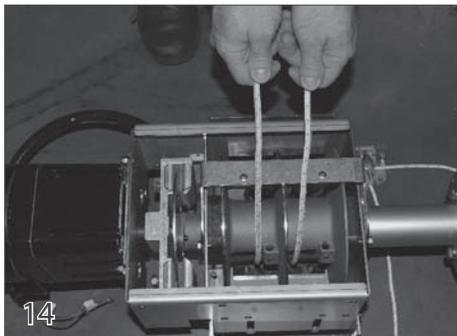
Pull the rope under the rope reel, over the rope containment bracket and out of the mechanism.
