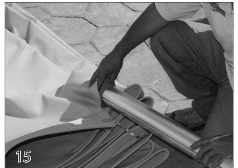
**Attaching The Cover Leading Edge** Lay the front of the cover in front of the mechanism. Slide the leading edge through the loop on the front of the cover.
