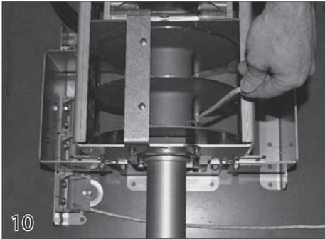
Direct this rope under the rope reel, over the rope containment bracket and out of the mechanism.
