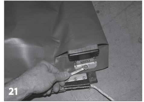
Tighten the nut (27) all the way down, then loosed 1/2 turn to allow movement between the slider and the leading edge insert. Repeat the installation of the leading edge insert on the other side of the cover.
