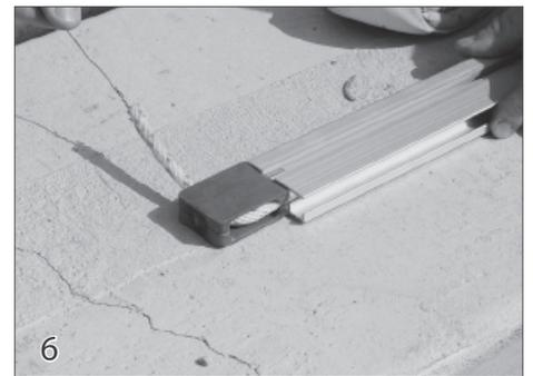
Feed the rope around the pulley end cap. (14)
