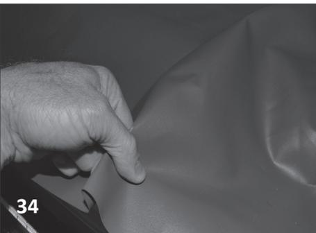
Find the center of the slack and pin directly to the tube (DO NOT FOLD THE SLACK). Repeat this step several times along the tube.
