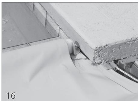
Feed one side of the cover and slider into the track. This will make it easier to insert in the leading edge tube.
