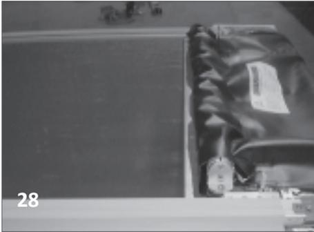
Pull the cover all the way open until the sliders stop against the guide feeds.
