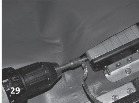
Attach the bonding wire to the leading edge bar using a self-tapping screw (30).
