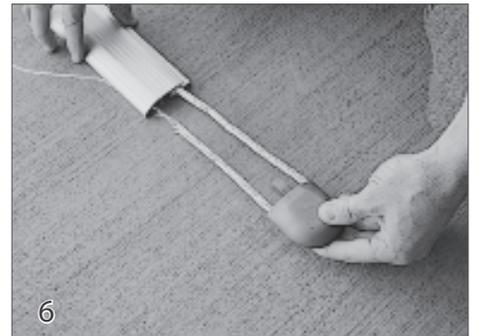
Feed the rope through the pulley assembly (28) and place the pulley housing onto the end of the track.
