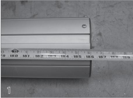
To determine if the cover system was ordered correctly for the pool, the length of the roll-up tube should be 3 inches shorter than the track space. For example, for an 16 foot track space, the correct length of roll-up tube is 15 ft 9 in.
