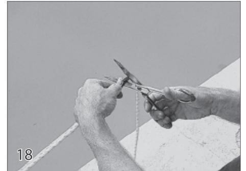
While pulling both ropes tight, use a lighter or torch to burn the rope in the location it will be cut. This will help them not fray after they have been cut. Cut the ropes so they are at least 8 ft long. Use the lighter to reburn the cut ends of the rope if needed.
