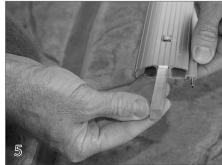
Tap the spring pin (46) into the round splice channel. Slide the center splice (45) into the center channel.
