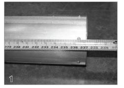
To determine if the cover system was ordered correctly for the pool, the length of the roll-up tube should be 3 inches shorter than the track space.
