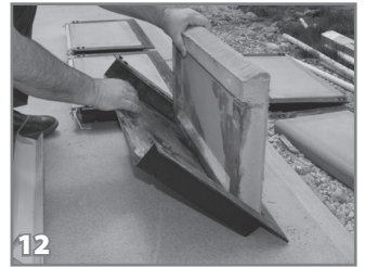
12 After the concrete is completely set, remove each lid section from the tray. Clean the trays and form pieces so they are ready for their next use.
