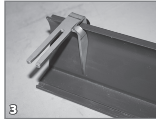
3 The lid forming retainer bracket comes in two options, one with a shape piece for the inclined or cantilever shapes, and one without the shape piece that is used with the vertical form.
