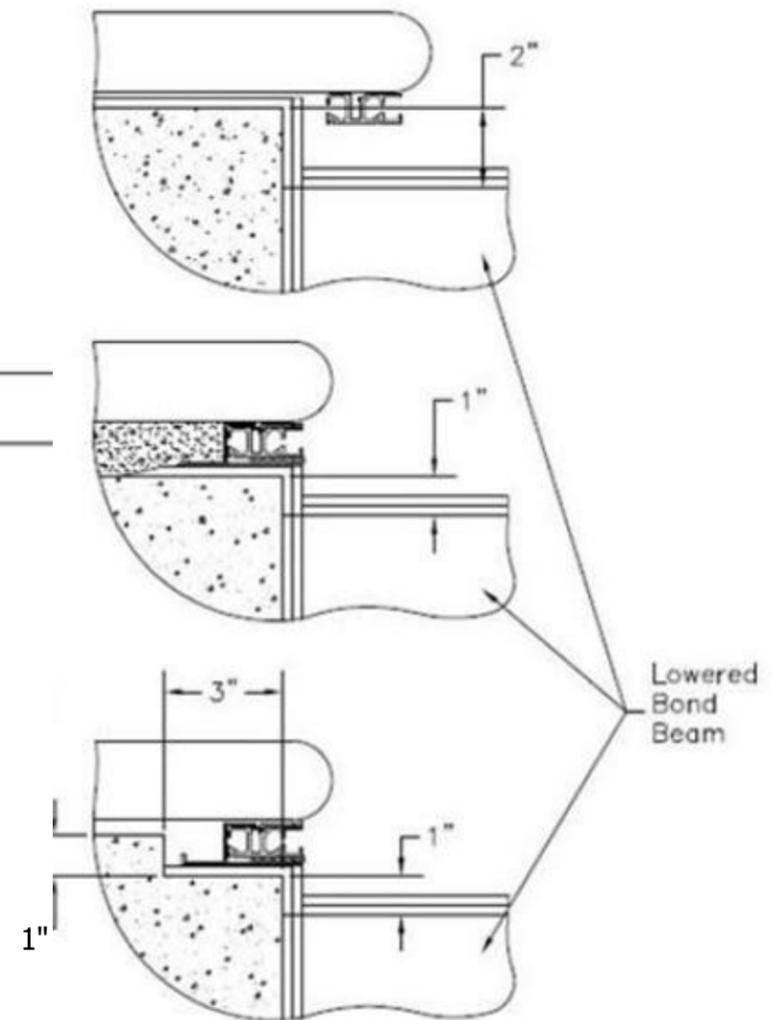
Concrete cover housing may be shaped and formed free hand or shot around a form. Walls must be straight and plumb, make housings square to pool. Steel cover housing walls same as pool. Do not allow rebound to be used for housing walls.
