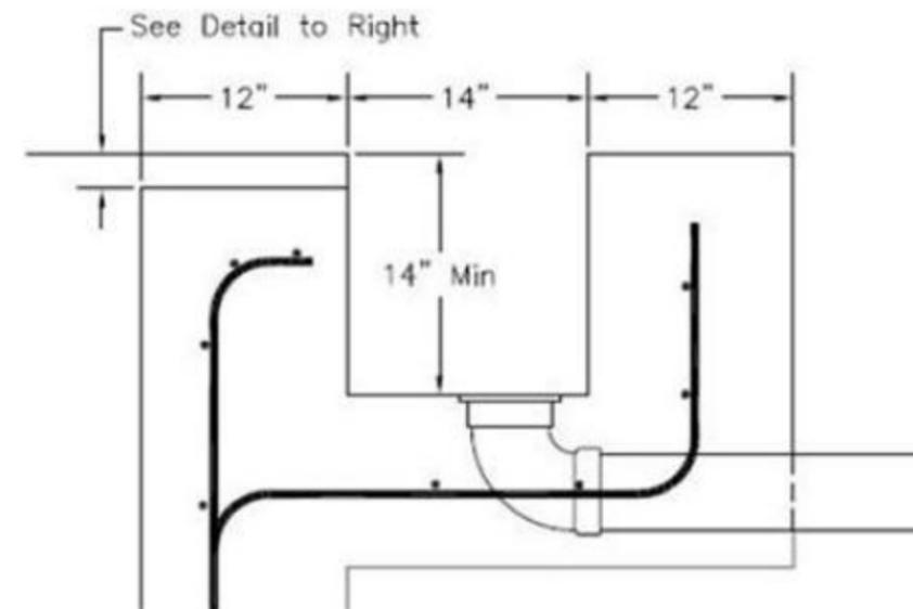
Because coping and deck thickness vary, housing depth is always measured from the top of beam or top of encapsulation.
